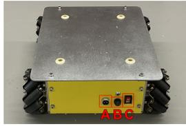
Fig. 2: Original Hangfa Discovery Q2 mobile platform (A: recharger socket; B: power fuse; C: power switch).
